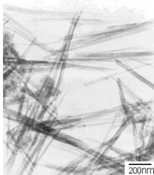
Fig. 3. TEM image of original attapulgite.
